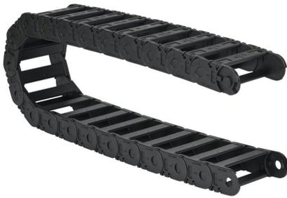
igus 2500 cable drag chain, 0.98in inside height, 3.03in inside width, 2.95in bend radius, outside opening, 1.81in pitch, 3.2ft/1m length, black. Requires 2070-34PZB or 2070-12PZB brackets for mounting.
