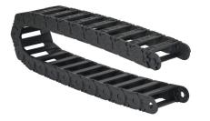
igus 2500 cable drag chain, 0.98in inside height, 3.03in inside width, 2.16in bend radius, outside opening, 1.81in pitch, 3.2ft/1m length, black. Requires 2070-34PZB or 2070-12PZB brackets for mounting.
