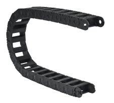
igus 2500 cable drag chain, 0.98in inside height, 2.24in inside width, 4.92in bend radius, outside opening, 1.81in pitch, 3.2ft/1m length, black. Requires 2050-34PZB or 2050-12PZB brackets for mounting.
