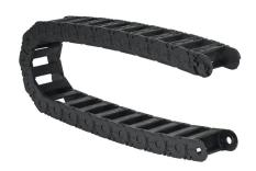
igus 2500 cable drag chain, 0.98in inside height, 2.24in inside width, 2.95in bend radius, outside opening, 1.81in pitch, 3.2ft/1m length, black. Requires 2050-34PZB or 2050-12PZB brackets for mounting.
