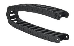
igus 2500 cable drag chain, 0.98in inside height, 2.24in inside width, 2.16in bend radius, outside opening, 1.81in pitch, 3.2ft/1m length, black. Requires 2050-34PZB or 2050-12PZB brackets for mounting.
