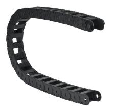
igus 2500 cable drag chain, 0.98in inside height, 1.5in inside width, 4.92in bend radius, outside opening, 1.81in pitch, 3.2ft/1m length, black. Requires 2030-34PZB or 2030-12PZB brackets for mounting.
