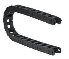
igus 2500 cable drag chain, 0.98in inside height, 1.5in inside width, 3.94in bend radius, outside opening, 1.81in pitch, 3.2ft/1m length, black. Requires 2030-34PZB or 2030-12PZB brackets for mounting.
