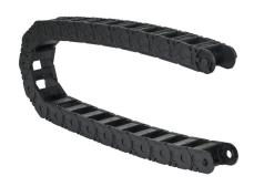
igus 2500 cable drag chain, 0.98in inside height, 1.5in inside width, 2.95in bend radius, outside opening, 1.81in pitch, 3.2ft/1m length, black. Requires 2030-34PZB or 2030-12PZB brackets for mounting.
