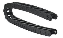
igus 2500 cable drag chain, 0.98in inside height, 1.5in inside width, 2.16in bend radius, outside opening, 1.81in pitch, 3.2ft/1m length, black. Requires 2030-34PZB or 2030-12PZB brackets for mounting.
