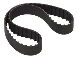
SureMotion timing belt, 3/8in L pitch, 1in wide, 65 tooth, 24.4in pitch length (circumference), neoprene, fiberglass reinforced.
