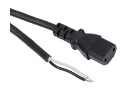
Stego heater connection cable, IEC320 C17 female power insert to pigtail, 6.5ft/2m cable length. For use with 0320xx-0x 1000W compact PTC fan heaters.
