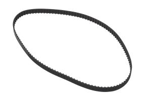
SureMotion timing belt, 1/5in XL pitch, 3/8in wide, 120 tooth, 24in pitch length (circumference), neoprene, fiberglass reinforced.
