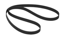
SureMotion timing belt, 0.08in MXL pitch, 1/4in wide, 240 tooth, 19.2in pitch length (circumference), neoprene, fiberglass reinforced. Package of 3.
