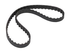
SureMotion timing belt, 3/8in L pitch, 1/2in wide, 64 tooth, 24in pitch length (circumference), neoprene, fiberglass reinforced.
