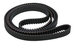
SureMotion timing belt, 8mm 8M pitch, 20mm wide, 300 tooth, 2400mm pitch length (circumference), neoprene, fiberglass reinforced.
