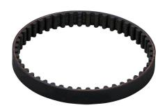
SureMotion timing belt, 5mm 5M pitch, 9mm wide, 48 tooth, 240mm pitch length (circumference), neoprene, fiberglass reinforced.
