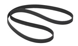
SureMotion timing belt, 0.08in MXL pitch, 1/4in wide, 236 tooth, 18.9in pitch length (circumference), neoprene, fiberglass reinforced. Package of 3.
