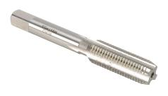
RUKO hand tap, M8 x 1.0 fine, square shank per DIN 10, high-speed steel (HSS), bright finish.
