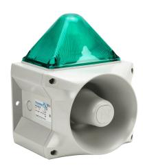
Pfannenberg PATROL series Xenon tube audible-visual signal beacon, 122 dB at 1m, (80) selectable tone(s), flashing strobe (1 Hz flash frequency), green, 214 x 181 x 270mm, 24 VDC, IP66, NEMA 4/4X.
