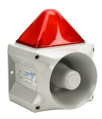
Pfannenberg PATROL series Xenon tube audible-visual signal beacon, 122 dB at 1m, (80) selectable tone(s), flashing strobe (1 Hz flash frequency), red, 214 x 181 x 270mm, 24 VDC, IP66, NEMA 4/4X.
