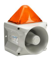
Pfannenberg PATROL series Xenon tube audible-visual signal beacon, 122 dB at 1m, (80) selectable tone(s), flashing strobe (1 Hz flash frequency), amber, 214 x 181 x 270mm, 24 VDC, IP66, NEMA 4/4X.
