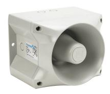
Pfannenberg PATROL series audible signal horn, 122 dB at 1m, 150 Hz to 2.9 kHz tone frequency, (80) selectable tone(s), 10-60 VDC, surface mount, ABS/polycarbonate housing, gray, IP66, NEMA 4/4X.
