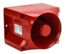
Pfannenberg PATROL series audible signal horn, 122 dB at 1m, 150 Hz to 2.9 kHz tone frequency, (80) selectable tone(s), 10-60 VDC, surface mount, ABS/polycarbonate housing, red, IP66, NEMA 4/4X.
