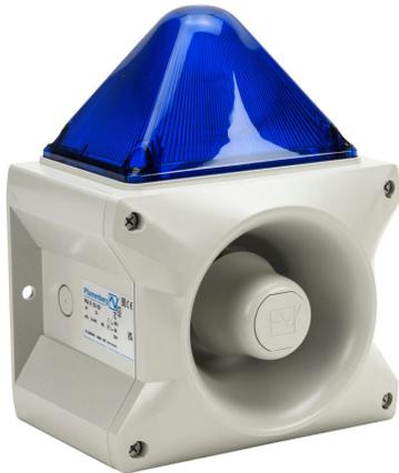
Pfannenberg PATROL series Xenon tube audible-visual signal beacon, 117 dB at 1m, (80) selectable tone(s), flashing strobe (1 Hz flash frequency), blue, 214 x 156 x 270mm, 24 VDC, IP66, NEMA 4/4X.
