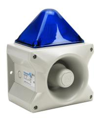
Pfannenberg PATROL series Xenon tube audible-visual signal beacon, 117 dB at 1m, (80) selectable tone(s), flashing strobe (1 Hz flash frequency), blue, 214 x 156 x 270mm, 24 VDC, IP66, NEMA 4/4X.
