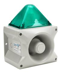
Pfannenberg PATROL series Xenon tube audible-visual signal beacon, 117 dB at 1m, (80) selectable tone(s), flashing strobe (1 Hz flash frequency), green, 214 x 156 x 270mm, 24 VDC, IP66, NEMA 4/4X.
