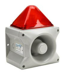
Pfannenberg PATROL series Xenon tube audible-visual signal beacon, 117 dB at 1m, (80) selectable tone(s), flashing strobe (1 Hz flash frequency), red, 214 x 156 x 270mm, 24 VDC, IP66, NEMA 4/4X.
