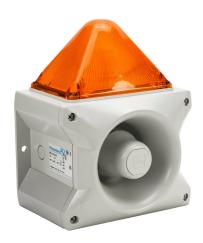
Pfannenberg PATROL series Xenon tube audible-visual signal beacon, 117 dB at 1m, (80) selectable tone(s), flashing strobe (1 Hz flash frequency), amber, 214 x 156 x 270mm, 24 VDC, IP66, NEMA 4/4X.
