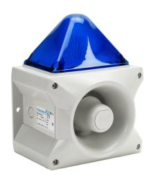
Pfannenberg PATROL series Xenon tube audible-visual signal beacon, 117 dB at 1m, (80) selectable tone(s), flashing strobe (1 Hz flash frequency), blue, 214 x 156 x 270mm, 115 VAC, IP66, NEMA 4/4X.
