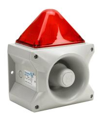
Pfannenberg PATROL series Xenon tube audible-visual signal beacon, 117 dB at 1m, (80) selectable tone(s), flashing strobe (1 Hz flash frequency), red, 214 x 156 x 270mm, 115 VAC, IP66, NEMA 4/4X.
