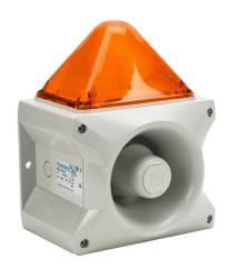
Pfannenberg PATROL series Xenon tube audible-visual signal beacon, 117 dB at 1m, (80) selectable tone(s), flashing strobe (1 Hz flash frequency), amber, 214 x 156 x 270mm, 115 VAC, IP66, NEMA 4/4X.
