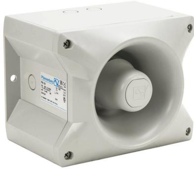
Pfannenberg PATROL series audible signal horn, 117 dB at 1m, 150 Hz to 2.9 kHz tone frequency, (80) selectable tone(s), 95-265 VAC, surface mount, ABS/polycarbonate housing, gray, IP66, NEMA 4/4X.
