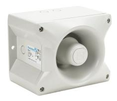
Pfannenberg PATROL series audible signal horn, 117 dB at 1m, 150 Hz to 2.9 kHz tone frequency, (80) selectable tone(s), 10-60 VDC, surface mount, ABS/polycarbonate housing, gray, IP66, NEMA 4/4X.
