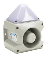
Pfannenberg PATROL series LED audible-visual signal beacon, 107 dB at 1m, (80) selectable tone(s), selectable permanent, blinking or flashing, red/yellow/green/blue, 163 x 132 x 215mm, 12-48 VDC, IP66, NEMA 4/4X.
