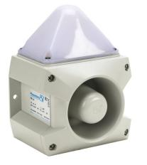
Pfannenberg PATROL series LED audible-visual signal beacon, 107 dB at 1m, (80) selectable tone(s), selectable permanent, blinking or flashing, red/yellow/green/blue, 163 x 132 x 215mm, 12-48 VDC, IP66, NEMA 4/4X.
