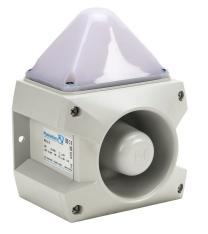
Pfannenberg PATROL series LED audible-visual signal beacon, 107 dB at 1m, (80) selectable tone(s), selectable permanent, blinking or flashing, red/yellow/green/blue, 163 x 132 x 215mm, 230 VAC, IP66, NEMA 4/4X.
