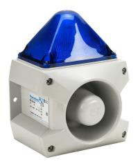
Pfannenberg PATROL series Xenon tube audible-visual signal beacon, 107 dB at 1m, (80) selectable tone(s), flashing strobe (1 Hz flash frequency), blue, 163 x 132 x 215mm, 24 VDC, IP66, NEMA 4/4X.
