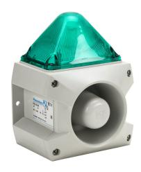
Pfannenberg PATROL series Xenon tube audible-visual signal beacon, 107 dB at 1m, (80) selectable tone(s), flashing strobe (1 Hz flash frequency), green, 163 x 132 x 215mm, 24 VDC, IP66, NEMA 4/4X.
