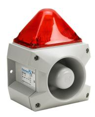
Pfannenberg PATROL series Xenon tube audible-visual signal beacon, 107 dB at 1m, (80) selectable tone(s), flashing strobe (1 Hz flash frequency), red, 163 x 132 x 215mm, 24 VDC, IP66, NEMA 4/4X.
