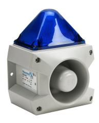
Pfannenberg PATROL series Xenon tube audible-visual signal beacon, 107 dB at 1m, (80) selectable tone(s), flashing strobe (1 Hz flash frequency), blue, 163 x 132 x 215mm, 115 VAC, IP66, NEMA 4/4X.
