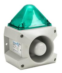
Pfannenberg PATROL series Xenon tube audible-visual signal beacon, 107 dB at 1m, (80) selectable tone(s), flashing strobe (1 Hz flash frequency), green, 163 x 132 x 215mm, 115 VAC, IP66, NEMA 4/4X.
