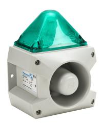
Pfannenberg PATROL series Xenon tube audible-visual signal beacon, 107 dB at 1m, (80) selectable tone(s), flashing strobe (1 Hz flash frequency), green, 163 x 132 x 215mm, 115 VAC, IP66, NEMA 4/4X.
