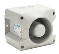
Pfannenberg PATROL series audible signal horn, 107 dB at 1m, 150 Hz to 2.9 kHz tone frequency, (80) selectable tone(s), 115 VAC, surface mount, ABS/polycarbonate housing, gray, IP66, NEMA 4/4X.
