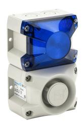
Pfannenberg PATROL series Xenon tube audible-visual signal beacon, 105 dB at 1m, (80) selectable tone(s), flashing strobe (1 Hz flash frequency), blue, 109 x 81 x 172mm, 24 VDC, IP66, NEMA 4/4X.
