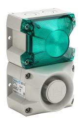
Pfannenberg PATROL series Xenon tube audible-visual signal beacon, 105 dB at 1m, (80) selectable tone(s), flashing strobe (1 Hz flash frequency), green, 109 x 81 x 172mm, 24 VDC, IP66, NEMA 4/4X.
