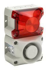
Pfannenberg PATROL series Xenon tube audible-visual signal beacon, 105 dB at 1m, (80) selectable tone(s), flashing strobe (1 Hz flash frequency), red, 109 x 81 x 172mm, 24 VDC, IP66, NEMA 4/4X.
