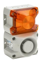
Pfannenberg PATROL series Xenon tube audible-visual signal beacon, 105 dB at 1m, (80) selectable tone(s), flashing strobe (1 Hz flash frequency), amber, 109 x 81 x 172mm, 24 VDC, IP66, NEMA 4/4X.
