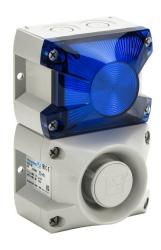
Pfannenberg PATROL series Xenon tube audible-visual signal beacon, 105 dB at 1m, (80) selectable tone(s), flashing strobe (1 Hz flash frequency), blue, 109 x 81 x 172mm, 115 VAC, IP66, NEMA 4/4X.
