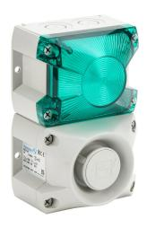
Pfannenberg PATROL series Xenon tube audible-visual signal beacon, 105 dB at 1m, (80) selectable tone(s), flashing strobe (1 Hz flash frequency), green, 109 x 81 x 172mm, 115 VAC, IP66, NEMA 4/4X.
