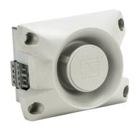
Pfannenberg PATROL series audible signal horn, 105 dB at 1m, 150 Hz to 2.9 kHz tone frequency, (80) selectable tone(s), 10-57 VDC, panel mount, ABS/polycarbonate housing, gray, IP66, NEMA 4/4X.
