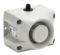
Pfannenberg PATROL series audible signal horn, 105 dB at 1m, 150 Hz to 2.9 kHz tone frequency, (80) selectable tone(s), 10-57 VDC, surface mount, ABS/polycarbonate housing, gray, IP66, NEMA 4/4X. Requires 4-pin female M12 cable.
