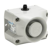
Pfannenberg PATROL series audible signal horn, 105 dB at 1m, 150 Hz to 2.9 kHz tone frequency, (80) selectable tone(s), 10-57 VDC, surface mount, ABS/polycarbonate housing, gray, IP66, NEMA 4/4X. Requires 4-pin female M12 cable.
