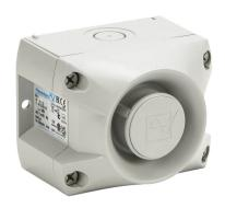
Pfannenberg PATROL series audible signal horn, 105 dB at 1m, 150 Hz to 2.9 kHz tone frequency, (80) selectable tone(s), 10-57 VDC, surface mount, ABS/polycarbonate housing, gray, IP66, NEMA 4/4X.
