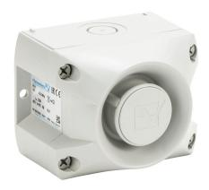
Pfannenberg PATROL series audible signal horn, 101 dB at 1m, 150 Hz to 2.9 kHz tone frequency, (80) selectable tone(s), 115 VAC, surface mount, ABS/polycarbonate housing, gray, IP66, NEMA 4/4X.
