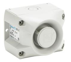
Pfannenberg PATROL series audible signal horn, 105 dB at 1m, 150 Hz to 2.9 kHz tone frequency, (80) selectable tone(s), 115 VAC, surface mount, ABS/polycarbonate housing, gray, IP66, NEMA 4/4X.
